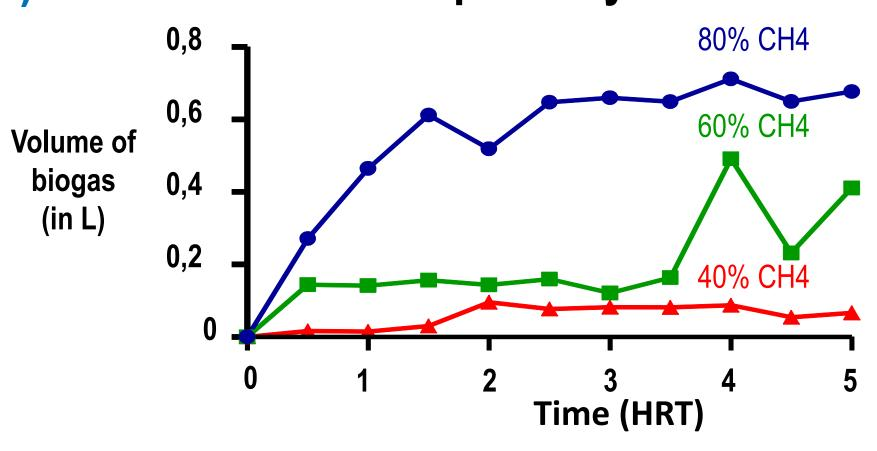
Biogas production over 100 days and methane proportion at steady state according to the origin of the inocula (soil, sediment, sludge) [5].
